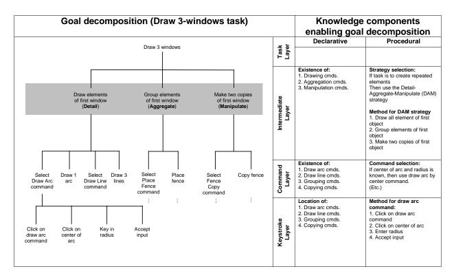
Figure 2. Cognitive analysis of the 3-window CAD task using the Detail-Aggregate-Manipulate strategy. The left part of the figure shows the hierarchical goal decomposition of the 3-window drawing task with the intermediate layer of knowledge marked in grey. The right part of the figure shows examples of the procedural and declarative components of knowledge at each layer of the decomposition that are required to complete the task.
